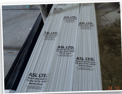
Bundles of PVC Trunking
